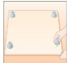
**2** Turn the base panel over so that it is standing on the legs. Using a screwdriver, screw four cam studs into the pre-drilled holes closest to each corner.
