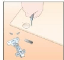
**4** Fix the hinges to the door using the screws provided. Make sure they are fitted squarely. Once all the hinges are in position on the door, fix them to the guide holes on the side panel of the cabinet. Do not over tighten the screws.
