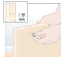
**5** Use a trimming knife to remove any excess edging at both ends of the grooves running along the length of the side panels. This is where the back panel will be fitted.
