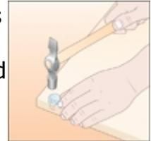
**3** To fit door hinges, use a bradawl to make guide holes in the pre-marked positions on the cabinet door. Insert the circular part of the hinge in the large hole in the door.
